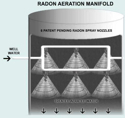
Rectangular Aeration Spray Manifold consisting of six (6) patent pending radon aeration nozzles.
