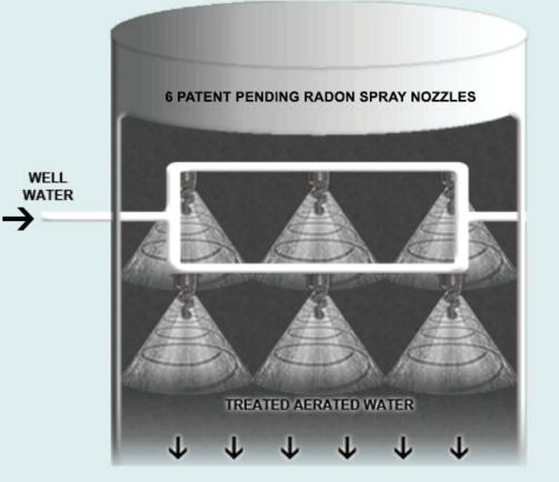
Rectangular Aeration Spray Manifold consisting of six (6) patent pending radon aeration nozzles.
